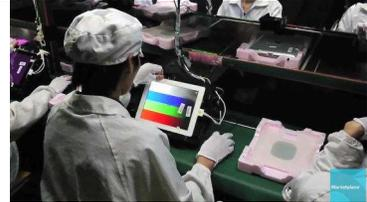
Final testing. No extended burn-in is required, probably because of the extensive ESD control and other quality control.
