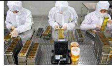
Bunny suits, gloves, ESD work surface and air ionizers for ESD protection.
